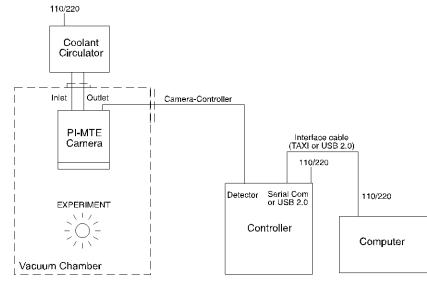
Figure 3. PI-MTE System Diagram
